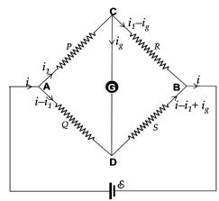
When the values of P, Q, R and S is so chosen that  $i_g = 0$ , the bridge is called '**balanced**'. In this condition, the potentials of C and D are the same and equations (i) and (ii) take the form,
