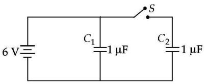
**Ans.** When the switch S is closed, the two capacitors in parallel will be charged by the same potential difference V.
