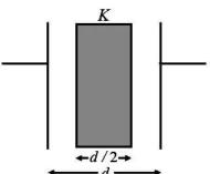
32. A capacitor, made of two parallel plates each of plate area A and separation d, is being charged by an external ac source. Show that the displacement current inside the capacitor is the same as the current charging the capacitor.  $[AI\ 2013]$
