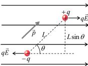
The forces acting on the poles (on the negative and the positive charges) are in opposite directions and equal to F = qE on each. But the distance between the
